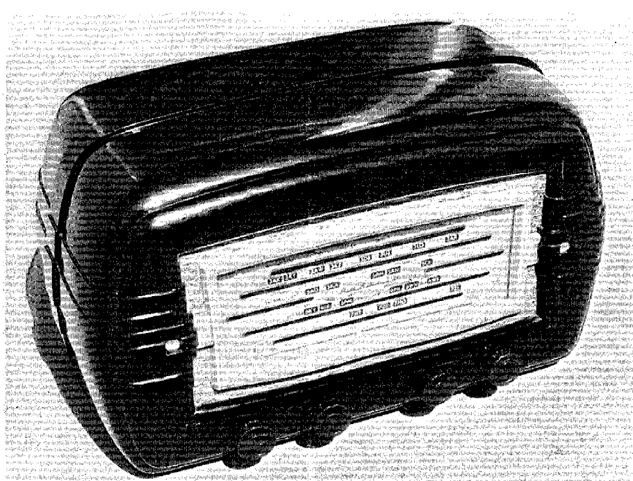
A Radiola with the rectangular dial escutcheon. This 4-valve model is unusual in that it is a dual-wave receiver. Very few 4-valve sets have a shortwave band.
