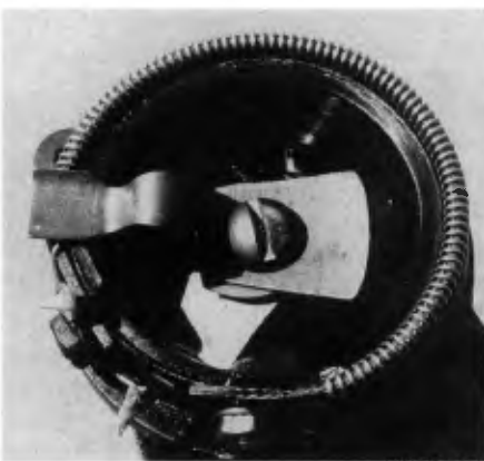
Because the low tension supply is unregulated, the supply voltage varies with the load. This wirewound rheostat is used to adjust the "A" voltage to suit the receiver.
