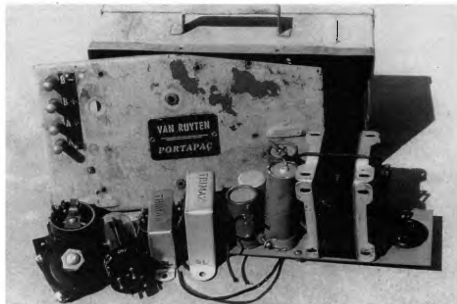
The old Van Ruyten battery eliminator is shown here stripped, ready for repairs. Like most vintage radio equipment it was in a fairly sorry state.
