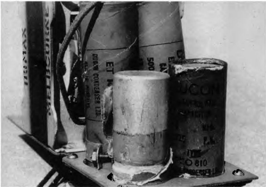
These old electrolytic capacitors were next to useless. Three had virtually no capacitance while the fourth had an internal short.
