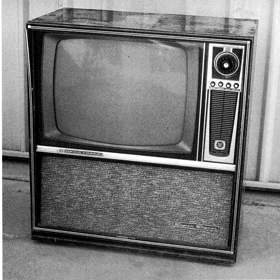
The AWA 242 was an up-market 21-inch set that was made during the mid 1960s. It had 21 valves and was fitted with a rotary VHF tuner.
