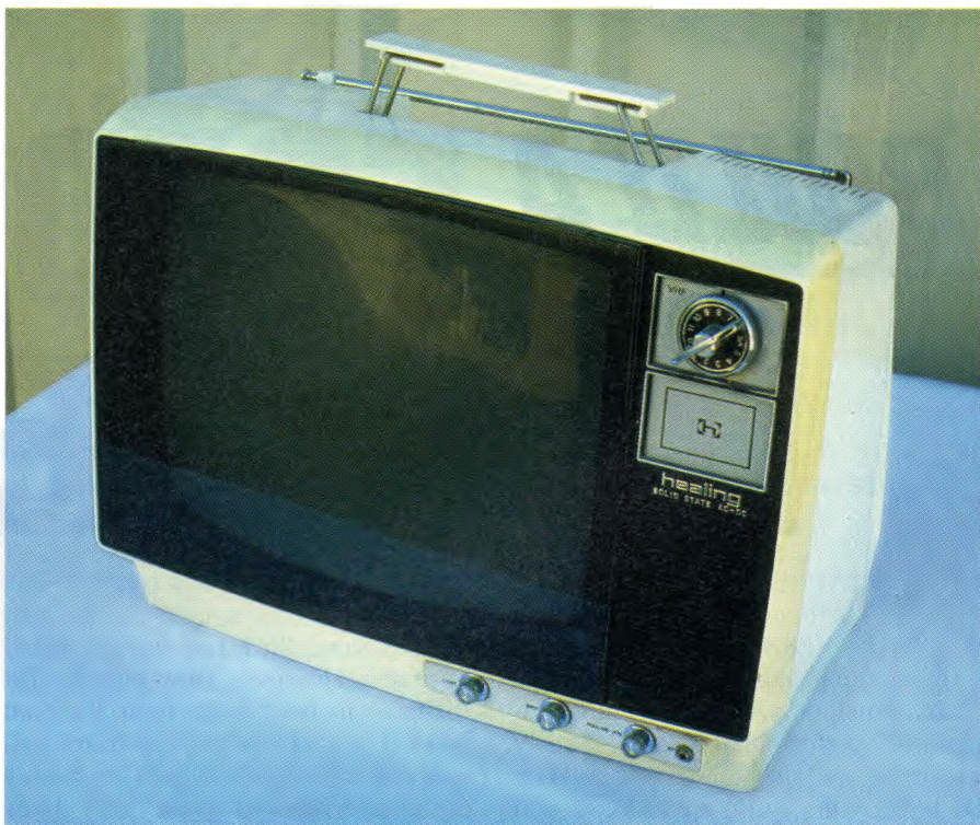
This portable b&w TV set carries the Healing brand name. It was made towards the end of the B&W era and uses solid state (transistorised) circuitry.
