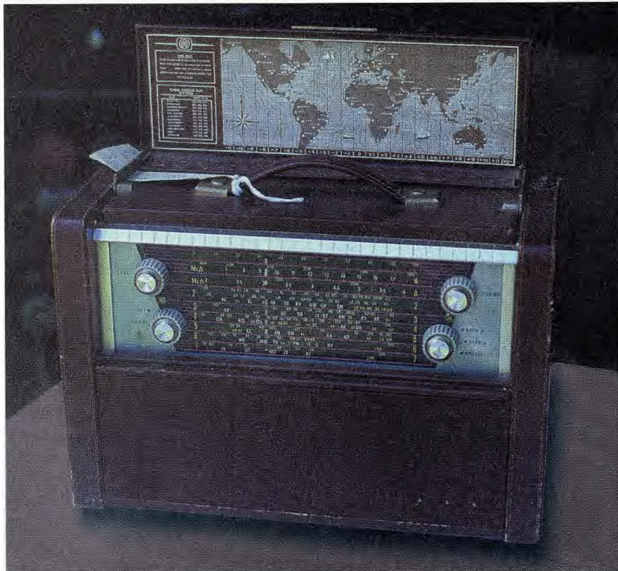
This multiband portable transistor radio included a flip-up lid with a world map that showed the locations of major shortwave stations.
