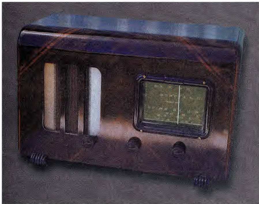
This home-made kitset mantel receiver (circa 1946) came in a stylish wooden case and has been fully restored. It featured inductance (Ferotune) tuning.
