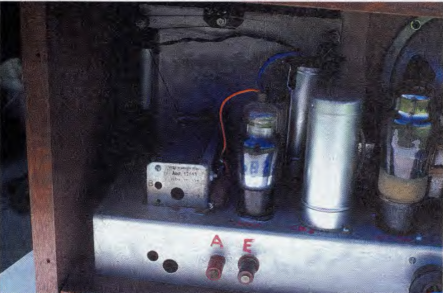
A close-up view of the Ferrotune inductance tuning module (at left), as used in the home-made receiver.
