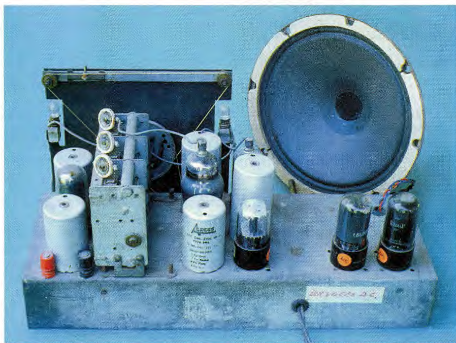
The chassis is easily removed from the cabinet for service, although the loudspeaker also has to be removed since its leads are too short.
