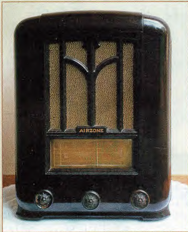
The Airzone Model 529: this was an AC/DC broadcast-band receiver with the following valve line-up: EK2 converter, CF2 RF amplifier, CBC1 detector/audio, CL2 output, CY2 rectifier and C1 ballast. (Photo courtesy Bill Adams, VK3ZWO).
