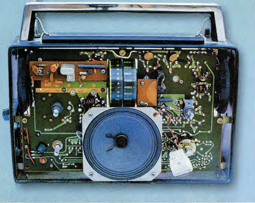
This view shows the front of the receiver with the front panel removed. The 1MHz crystal oscillator is shown at the top left of the photograph.
