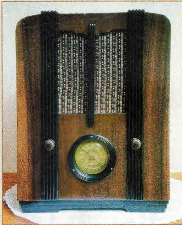
The Airzone Model 511: this AC broadcast-band model featured a circular dial and carried the following valves: 6A8 converter, 6K7 RF amplifier, 6Q7 detector/audio, 6F6 output and 5Z4 rectifier. (Photo courtesy Bill Adams, VK3ZWO).
