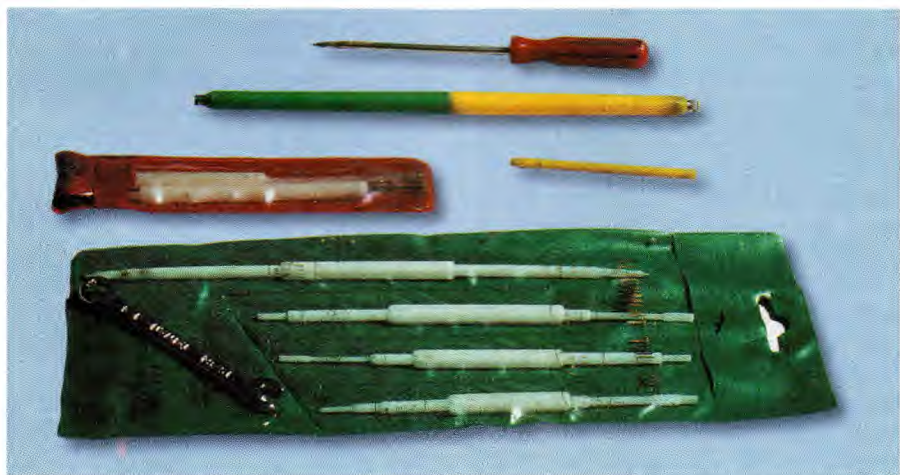
A selection of plastic alignment tools will be necessary if you intend restoring vintage receivers.
