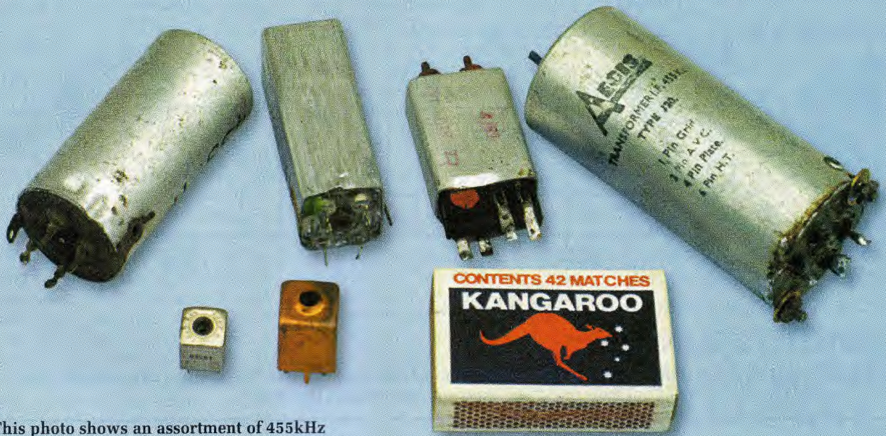
This photo shows an assortment of 455kHz IF transformers. They came in a wide range of sizes.
