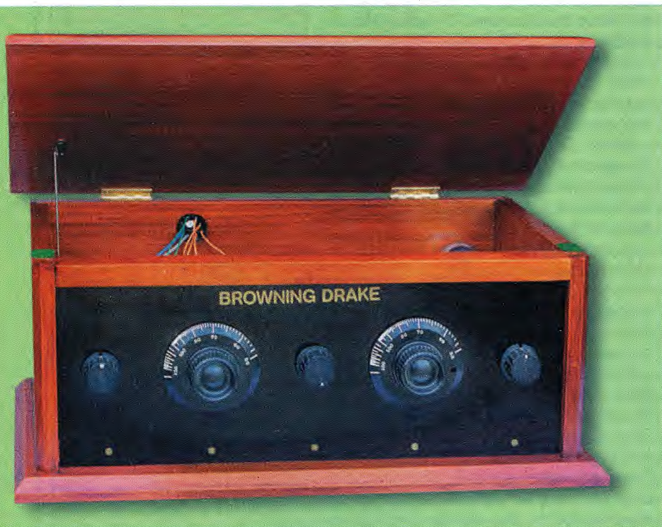
This view shows Jim Birtchnell’s completed Browning-Drake replica receiver. The hinged lid allows easy access to the circuit components.
