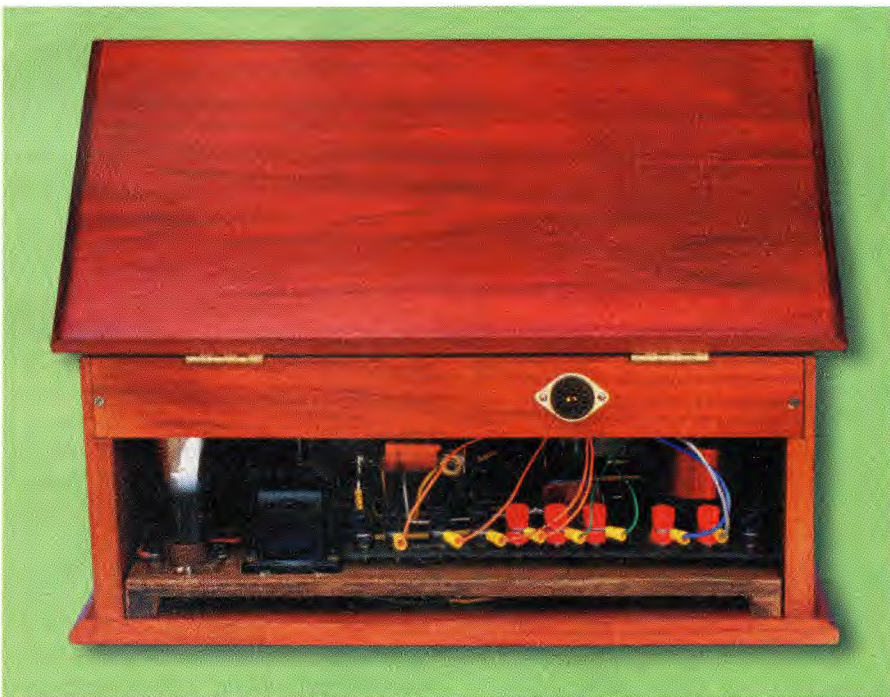
This rear view of set shows the antenna earth and power supply terminals. Note the power socket which allows an external supply to be connected.
