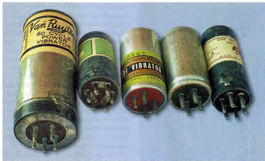
Five typical vibrators (from left to right): Van Ruyten 32V 200W dual interrupter vibrator, Oak V6606 6V dual interrupter (with strapped pins) vibrator, Oak V5124 6V synchronous vibrator, Plessey 121HD4 12V non-synchronous vibrator and Ferrocart M437 6V non-synchronous vibrator.
