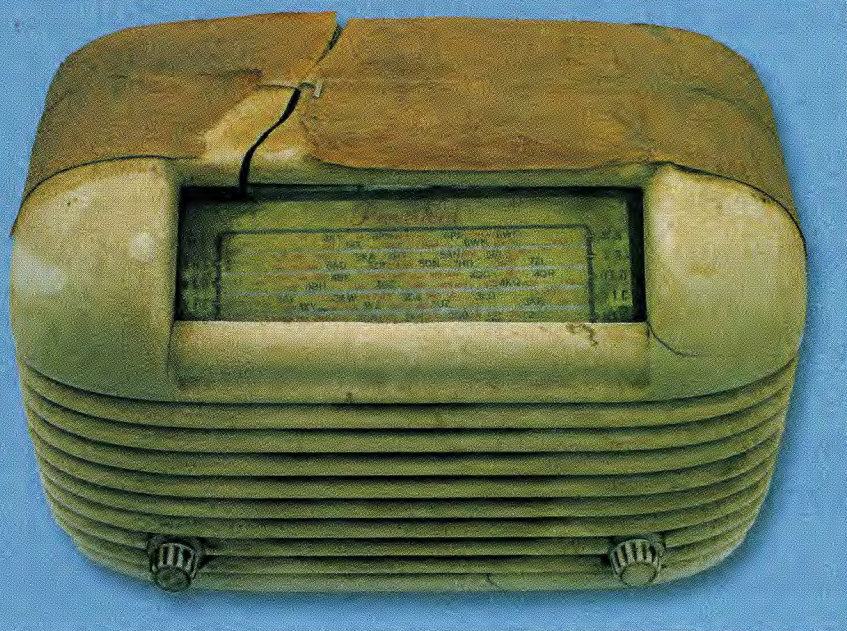
This is the 4-valve Precedent mantel set before restoration. Its cabinet had a bad crack at the top and was held together by masking tape.
