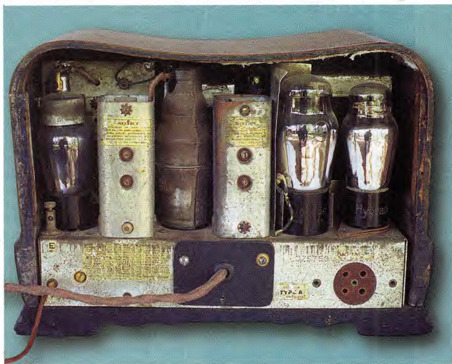
Below: a rear view of Astor OZ. This shows the very compact nature of the set, considering that it uses full-sized components. Be aware that a sheet of asbestos is used above the two valves at the right of the photograph. ▶
