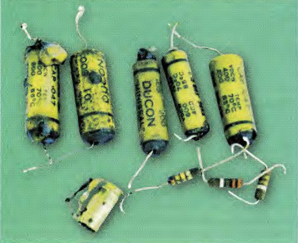
These are just some of the parts that were replaced in the set. It's a good idea to replace paper capacitors as a matter of course.
