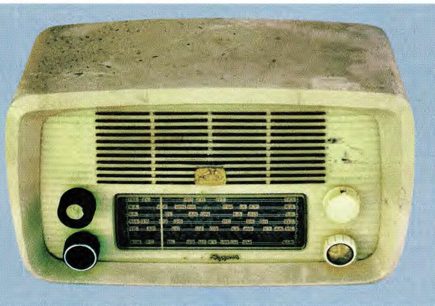
This view shows the Little Nipper receiver as it landed on my workbench. It was dirty and fitted with the wrong knobs - and that was just the outside.
