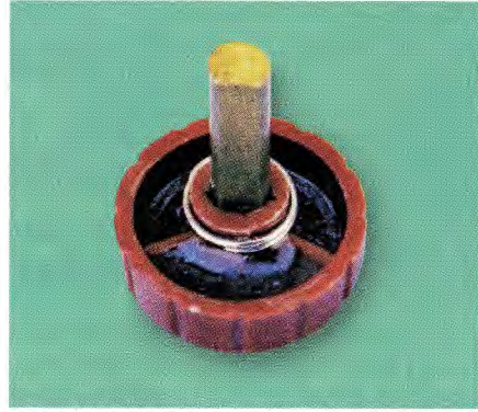
The Araldite is "poured" into the underside of the control knob, while the keyring prevents the centre boss from breaking again.
