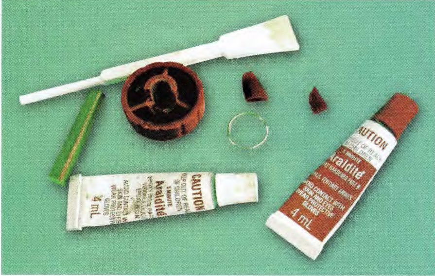
The control knobs can usually be repaired using Araldite (or a similar epoxy adhesive), a small key ring and a scrounged (greased) control shaft. The control shaft is removed after the Araldite has set.
