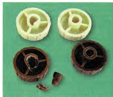
The original knobs fitted to the "Little Nipper" had a tendency to break in the centre.
