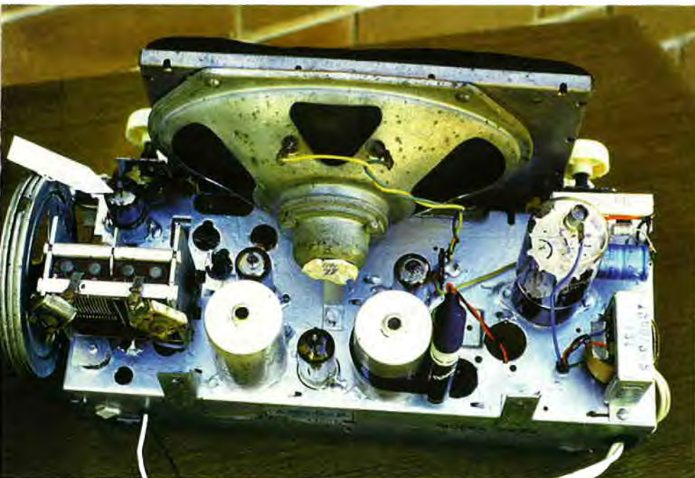
This view shows the chassis layout of the converted 32V receiver, with the white arrow (top left) indicating the new 6BA6 RF stage. A chassis photo of a similar main-powered version of this set is on page 81 of the September 2004 issue.
