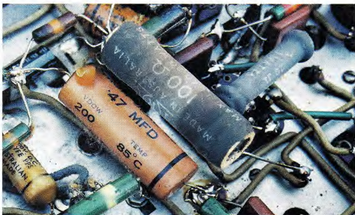
The old Monarch D671/32 was fitted with a gear driven tuning capacitor, as shown in the photo at left. The close-up above shows an overheated 0.47µF paper capacitor that's located too close to a high-wattage resistor.
