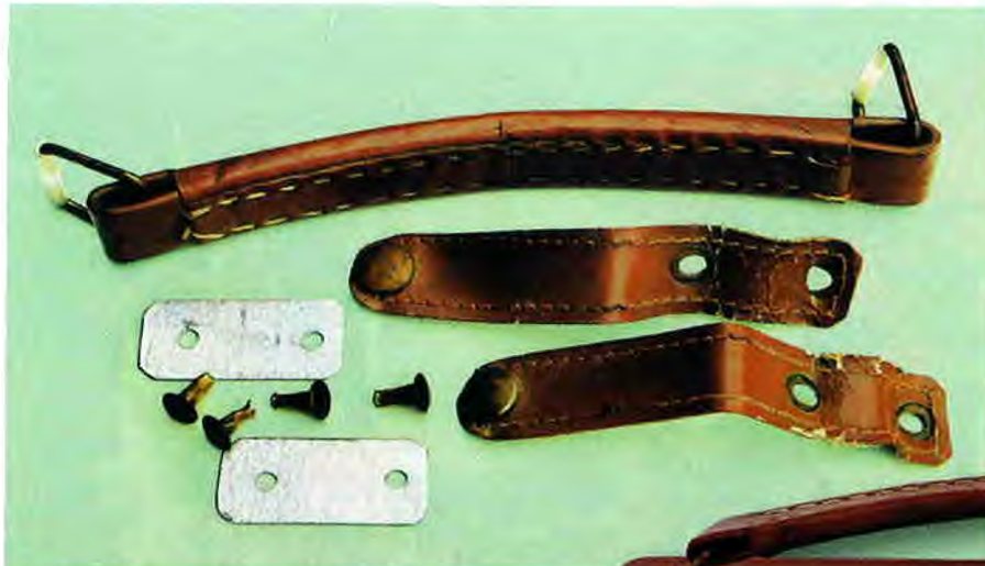
The handle assembly on the old B29 was repaired and strengthened using two small metal brackets (above and right). The restored receiver looks good and gives reasonable performance.
