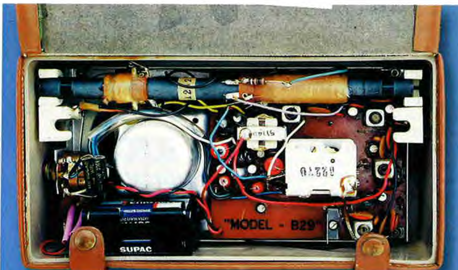
The original 2364 battery type used in the B29 is no longer available but six AA cells in a holder can be used instead.
