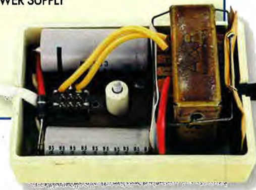
Fig.1: there's not much in the A&R PS82 battery eliminator – just a transformer, a diode, a couple of electrolytic capacitors and a switch to select the transformer taps.
