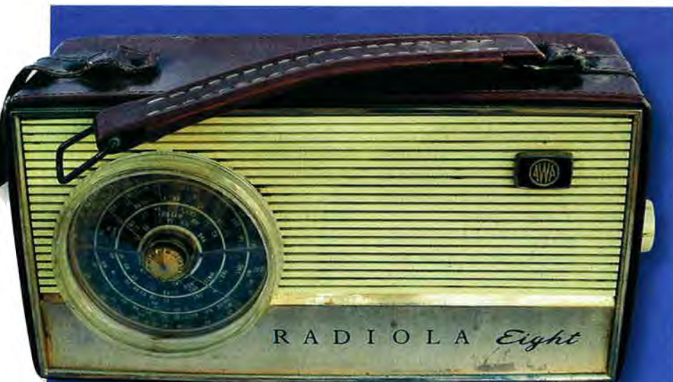
Although still functional, the old AWA Radiola B29 was somewhat worse for wear. It's a fairly conventional 8-transistor set from the 1960s.
