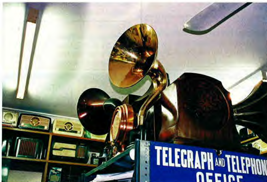
This view shows some of Brian's early horn and cone speakers. They date from around 1924 for the horn speakers to around 1928 for the moving-iron balanced-armature type cone speakers.
