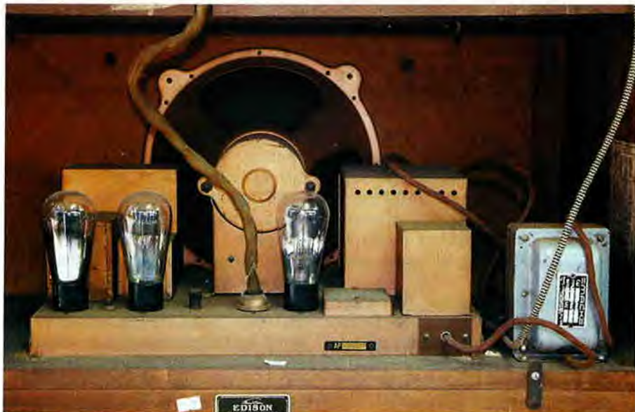
A close-up view of the audio output/power supply chassis and the large electrodynamic loudspeaker. The added 240V/115V transformer looks out of place.
