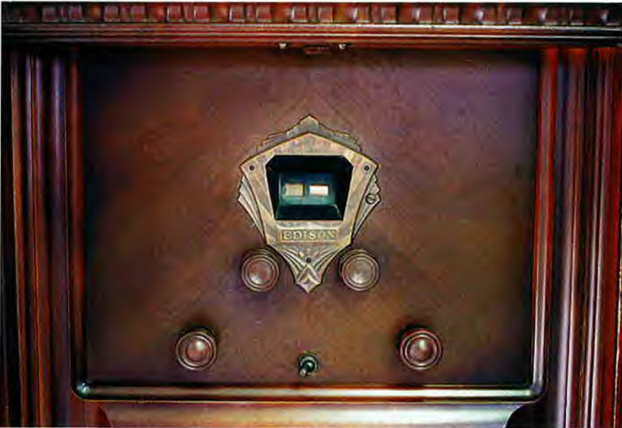
A close-up view of the Edison R6's control panel: from bottom left to right, volume, on/off and tone; and from top left to right, local/distance and tuning.
