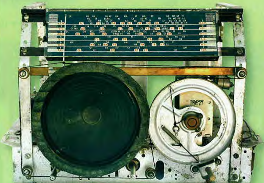
This view shows the front of the chassis after restoration. The dial-drum is driven by a rubber tyre assembly.
