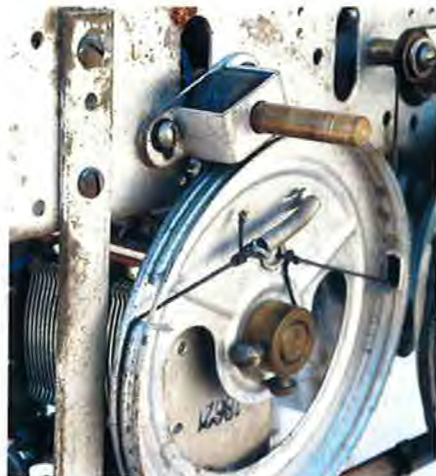
This close-up view shows the rubber tyre dial-drive system used on the B11A receiver.
