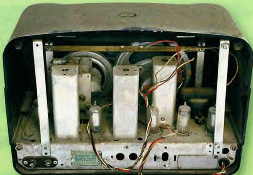
Despite its rather grubby condition, this set was relatively easy to restore as all the original parts were still in place. The chassis was cleaned by first dusting it with a paintbrush and then using a kerosene-soaked rag and a kitchen scourer.
