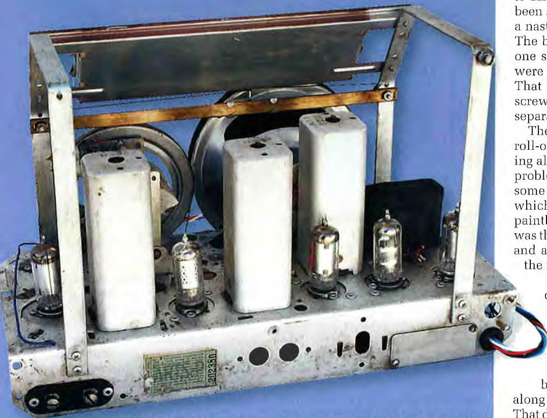
The chassis is fitted with a roll-over frame and can be tipped into any position for servicing without damaging other parts.
