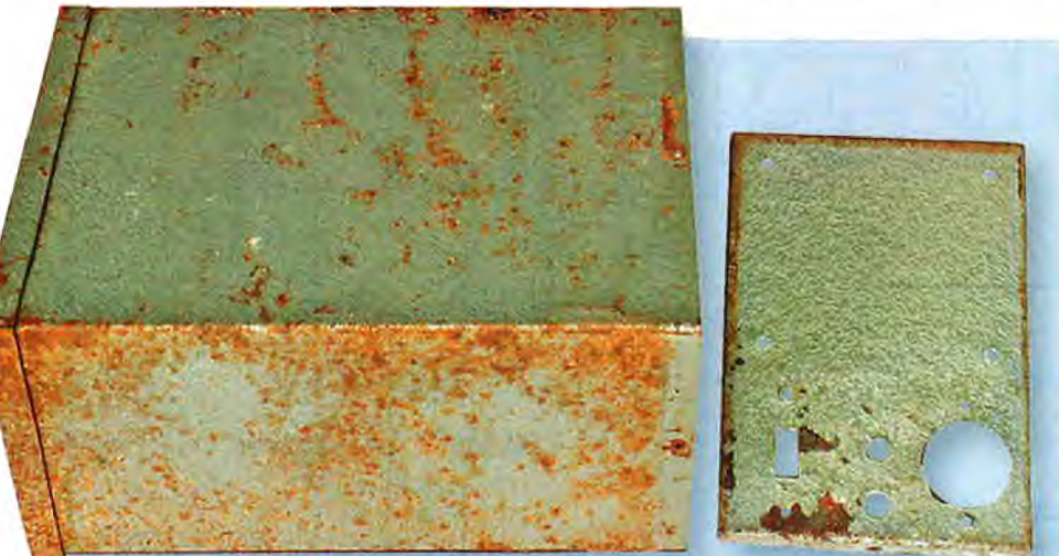
This is the Van Ruyten inverter's case before restoration. The rust was removed using a drill fitted with a wire brush, after which the unit was repainted so that it now looks almost like new.
