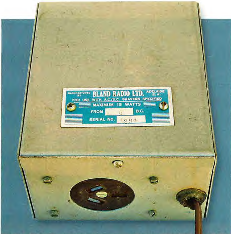
This simple 6V DC to 24VAC inverter was made by Bland Radio Ltd of Adelaide and was designed to power electric shavers.
