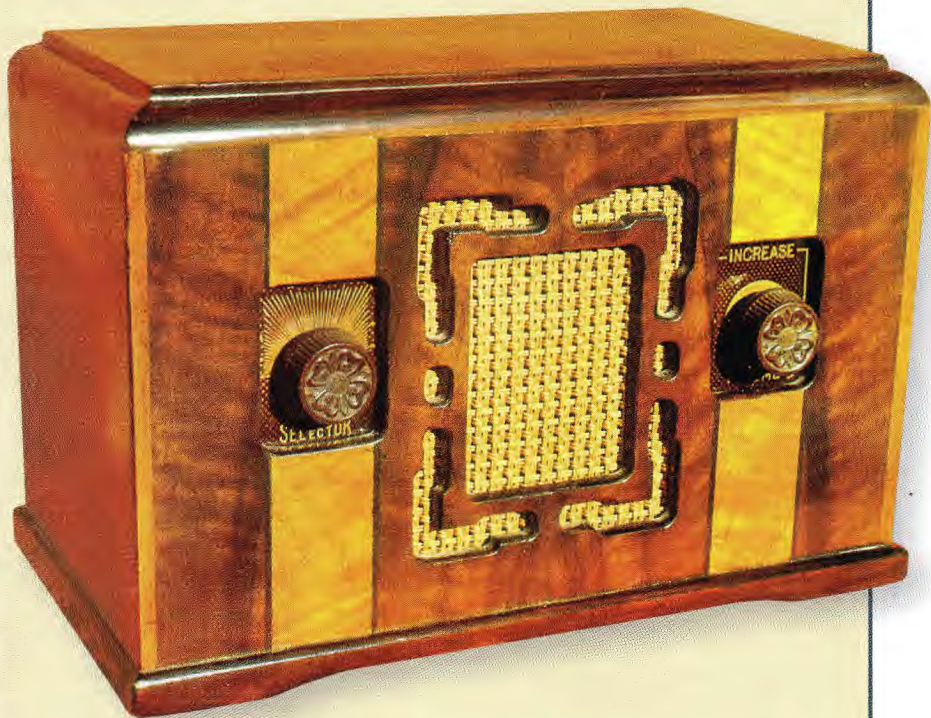
PRODUCED BY THE RACOPHONE COMPANY, SYDNEY , in 1933, the "Pee Wee" was a small 4-valve autodyne superhet receiver. It was housed in an attractive wooden cabinet and used the following valve types: 57 autodyne mixer; 57 anode bend detector; 2A5 audio output; and 80 rectifier. Photo: Historical Radio Society of Australia, Inc.
