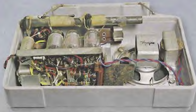
Removing the HT battery gives good access to the under-chassis parts in the Olympic #450. There's some chassis corrosion but the set is otherwise in good condition.
