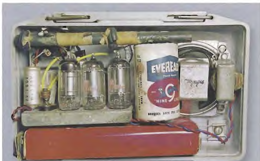
Inside the Olympic #450 4-valve miniature receiver. The ferrite rod antenna is similar to that used later in transistor radios.
