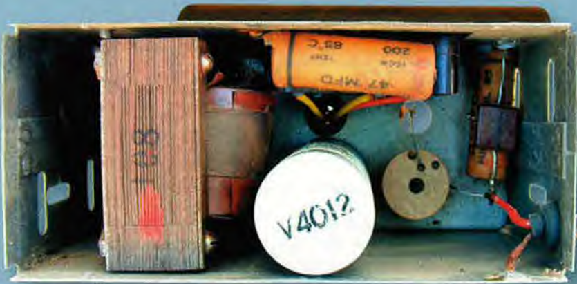
This is the view inside the Ferris inverter, from the top. The vibrator unit is located at bottom centre, immediately to the right of the transformer.
