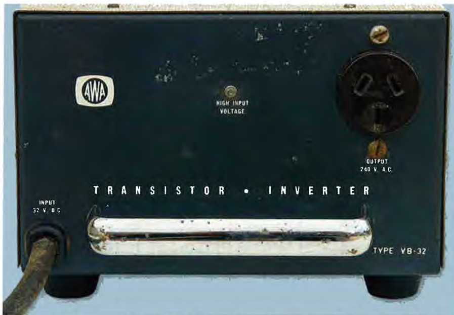
This is the AWA VB-32 inverter following restoration. It produced nominally 60-65Hz 240V AC at up to 180W from a supply of 32V DC.
