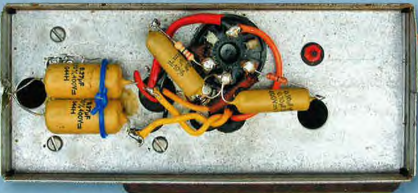
This view shows underside of the Ferris inverter after restoration. The paper capacitors were replaced with polyester units.
