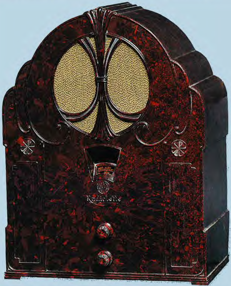
THE FIRST AUSTRALIAN RADIO IN A BAKELITE case was the AWA C87, launched in 1932. It was a 3-valve set and the valve line-up was as follows: 35 RF amplifier, regenerative 24 detector and 47 audio amplifier. This set is now one of the most sought-after by vintage radio collectors. Photo: Kevin Poulter, for the Historical Radio Society of Australia.
