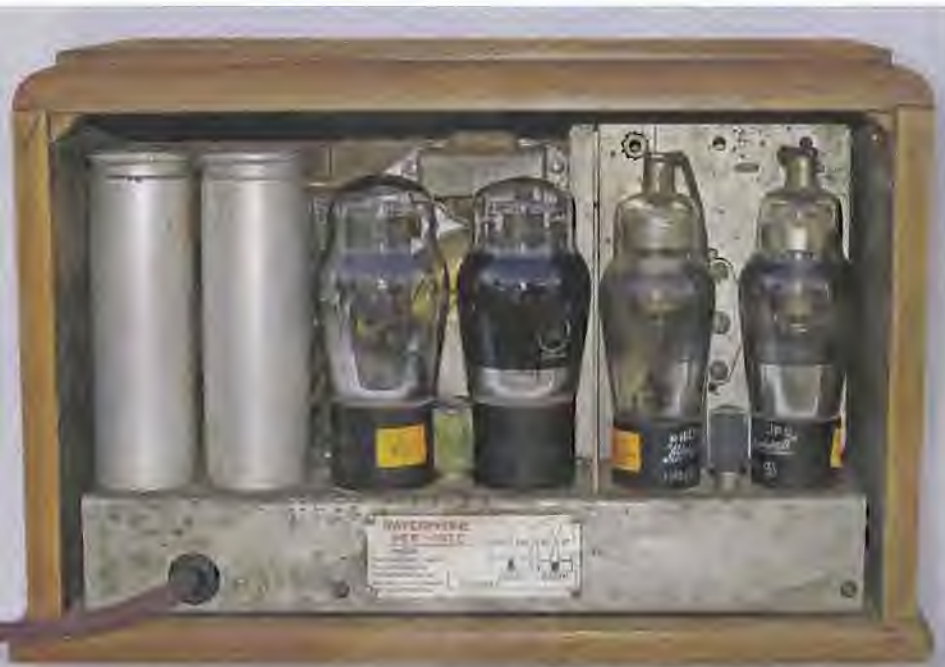
There's not much room left inside the cabinet when the chassis is slid into place, although the valves can still be replaced. Note the thickness of the timber used to make the cabinet.
