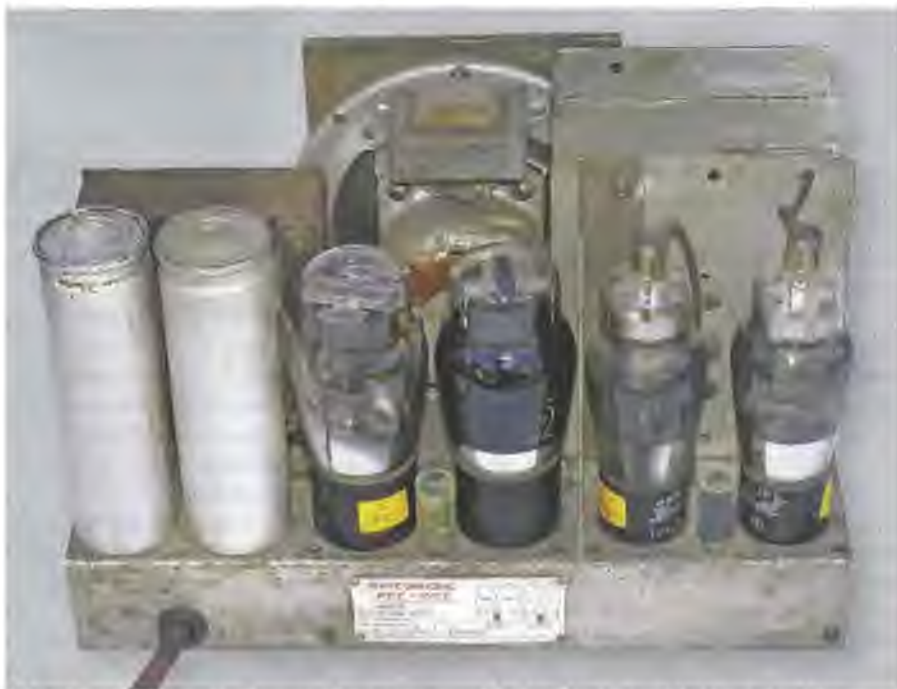
The chassis is easy to remove but care must be taken to avoid damaging the under-chassis components. The parts mounted on the top of the chassis are all easily accessible.
