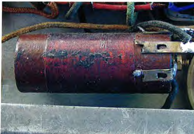
Left: a solenoid-type aerial coil as used in the Raycophone "Pee Wee" AM radio from about 1933.
