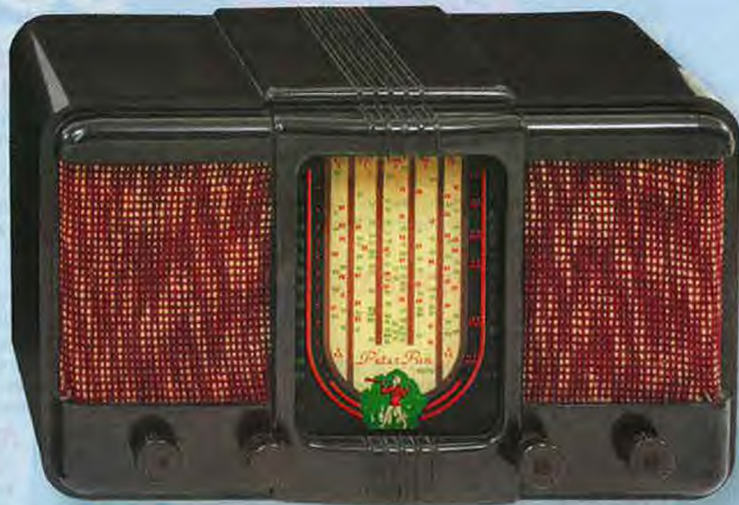
The Peter Pan BKJ was manufactured around 1946 by Eclipse Radio in Melbourne and this particular example was restored by Bill Smith. It employed a conventional superhet circuit and the valve line-up was as follows: 6J8G mixer, 6U7G IF amplifier, 6B6G detector/first audio amplifier, 6V6G audio output and 5Y5G rectifier. Photo by Kevin Poulter for the Historical Radio Society of Australia (HRSA). Phone (03) 9539 1117. www.hrsa.net.au
