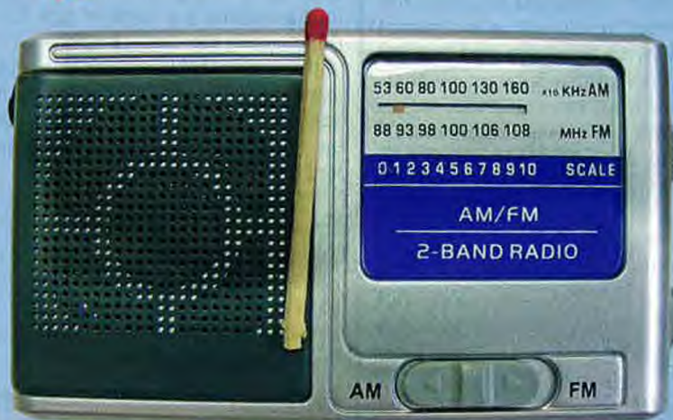
This small AM/FM receiver uses the PC board shown above and is intended for use in strong signal areas only. Its miniature ferrite rod antenna means that its AM performance is pathetic compared to larger sets.
