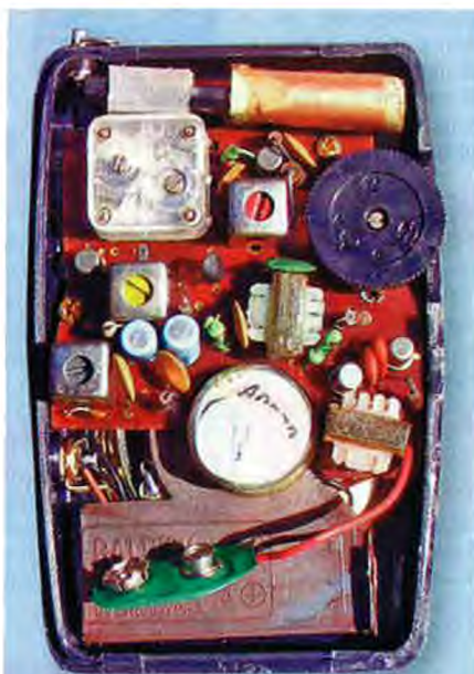
A typical "pocket-portable" AM radio from the 1970s. The small loopstick antenna is at the top and gave adequate performance on strong local stations.
