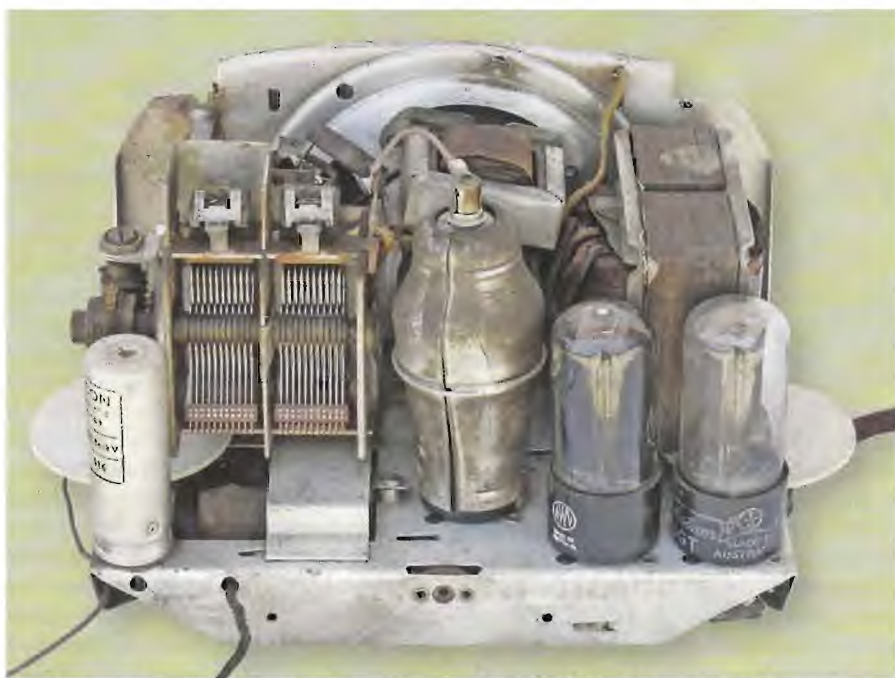
The above-chassis parts are close together but can be easily accessed once the valves have been removed. Note the metal shield on the 6G8G RF valve.
