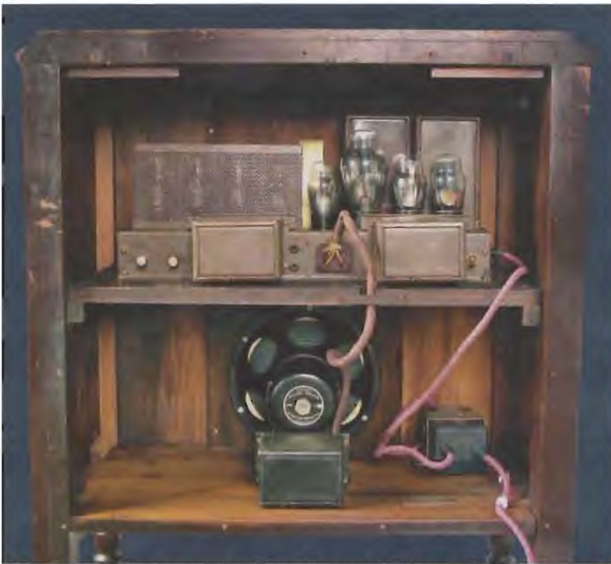
The chassis sits on a horizontal shelf in the top half of the cabinet, while the loudspeaker assembly is mounted in the bottom half and is connected via a cable and plug. Note the 240V to 110V step-down transformer at bottom right.
