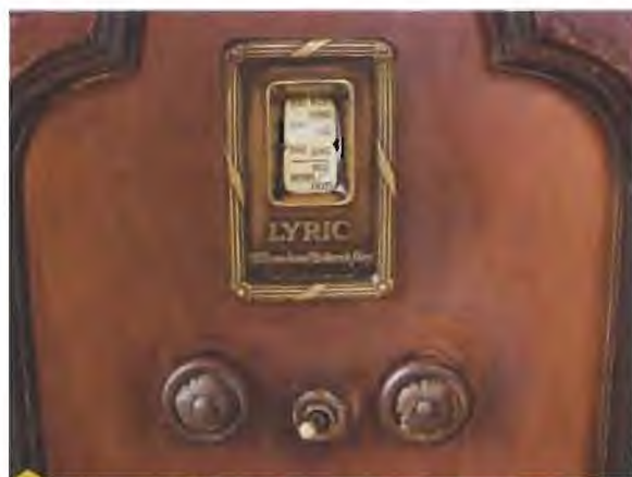
Above: the dial has both wavelength and kilocycle markings, while the Tuning and Volume controls are mounted directly beneath the dial escutcheon. The toggle switch in the centre is the On/Off control.
