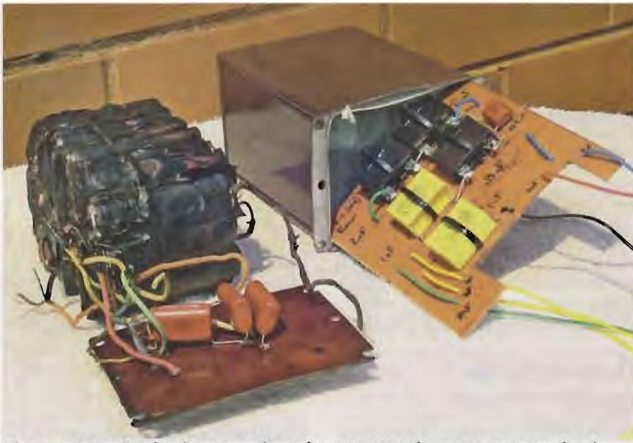
The new capacitor bank was made up by mounting the parts on a couple of pieces of fibreboard and connecting them via flying leads. This assembly was then housed in the original box. The original capacitor bank is visible at top left.
