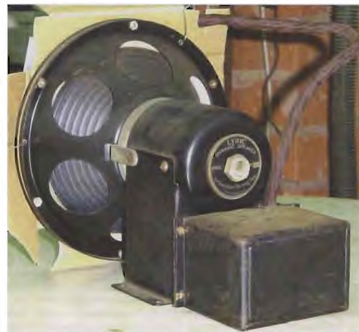
Left: the iron-cored chokes, the speaker transformer and the electrodynamic speaker are all attached to each other to form a single assembly. This assembly is connected via a cable and plug to the chassis.
