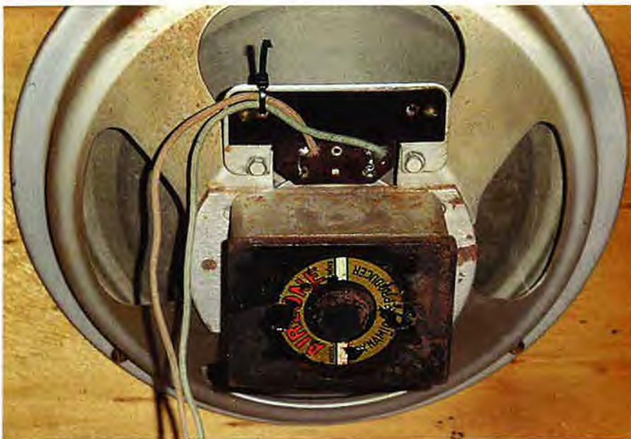
The original loudspeaker required some work to get it going again, including a patch on the paper cone. The flexible wires that connect the voice coil to the speaker transformer had also been damaged and required replacement.
