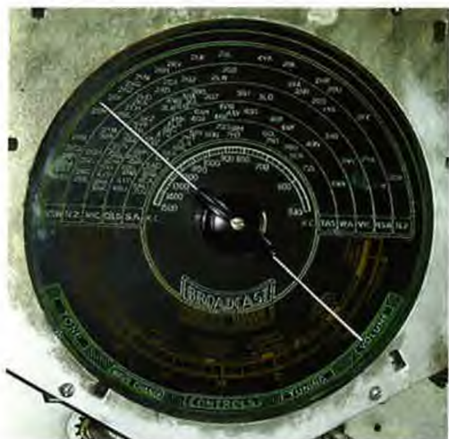
A close-up view of the dial scale. The dial lamps are switched so that only the broadcast or shortwave markings are illuminated.
