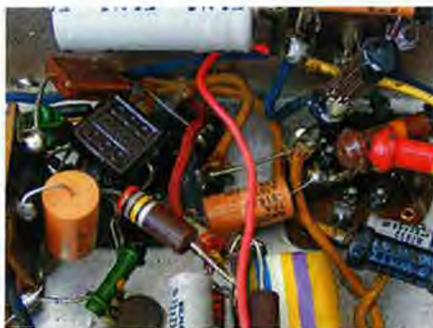
The parts around the detector/first audio amplifier socket are somewhat crowded together.
