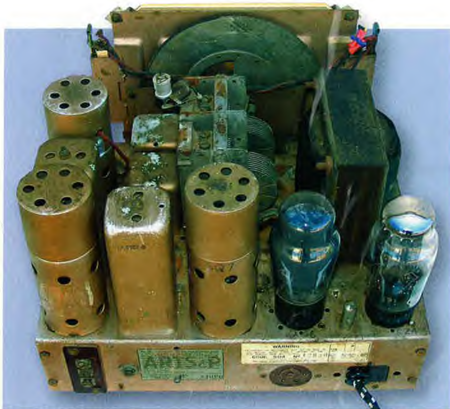
The top of the chassis is tightly packed with the major parts. Metal shields are fitted to the converter, IF and detector/triode valves, while the mains cord is now firmly anchored with a cordgrip grommet in place of the original knot.
