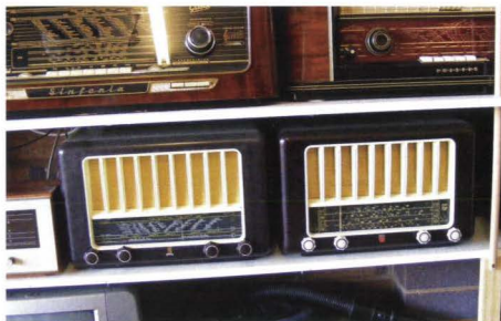
The Philips Sierra model H283 (left) and its Australian Philips equivalent. The cabinets are identical, although different dial scales are used to suit the intended market.
