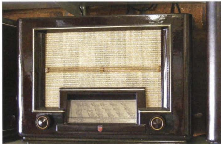
Despite being badly damaged in transit, this 1939 Philips BX480A has now been restored to full working order. The restoration included extensive cabinet repairs and the manufacture of a new glass dial-scale.
