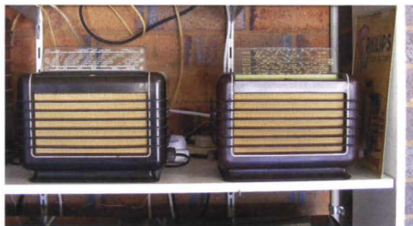
Another set of Philips twins, this time showing the Dutch model 209U and the visually identical Australian model 112 at right. Note the "pop-up" dial scales.
