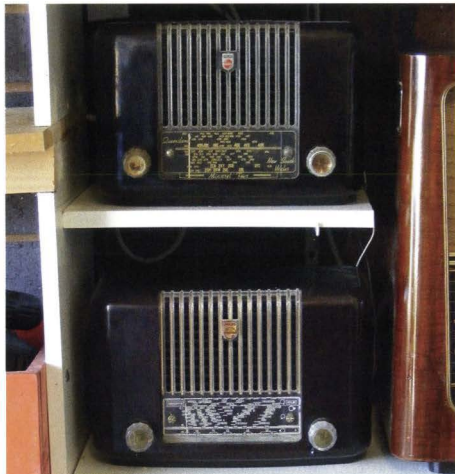
More Philips "twins" – the Australian model 138 is shown at top, while below it is the almost visually-identical Dutch BX221U.
