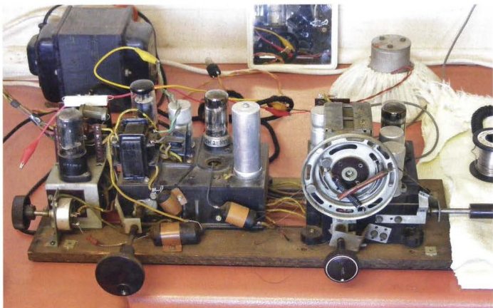
This view shows the three-part aluminium and Bakelite chassis of a Sierra 159X receiver which is currently undergoing restoration on John's workbench.
