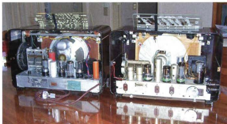
The Australian Philips 115 and the Dutch Philips BX462A from the rear, with their backs removed. The differences between the two chassis are quite marked.
