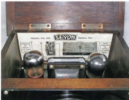
Inside of the Seyon receiver with the lid raised. The label attached to the rear panel shows how the batteries, antenna and earth are connected to the set.
