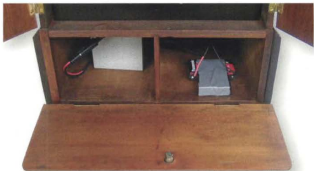
The batteries for the 1-valve set sit in a special battery compartment at the bottom of the cabinet.
