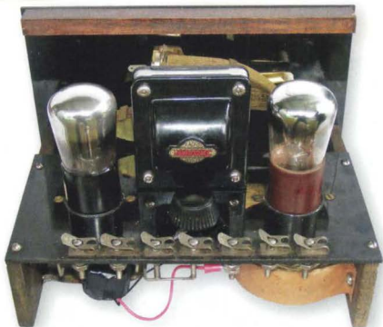
An above-chassis rear view of the 2-valve Seyon receiver. Note the large interstage audio transformer between the two valves and the row of spring terminals along the rear edge to terminate the battery connection leads.
