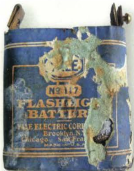
Despite its age, the original bias battery, a Yale flashlight type, still had an output of 1.3V.
