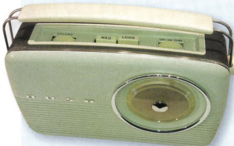
The TR82C's volume, wave-change and on-off/tone controls sit in a recessed well at the top of the case. A large dial "wheel" on the front of the set is used for tuning and is easy to operate.
