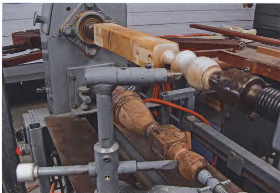
The author's home-made copy wood lathe came in handy when it came to making new sections for the turned legs that are fitted to the cabinet.
