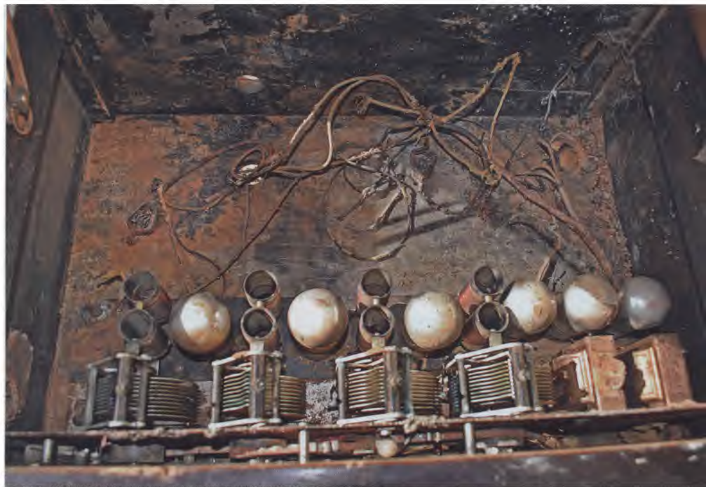
The 84-year-old AWA C54 was obtained by the author in very poor condition, with a badly water-damaged cabinet and a dirty, rusting chassis. Restoring it to full working condition was a monumental task.
