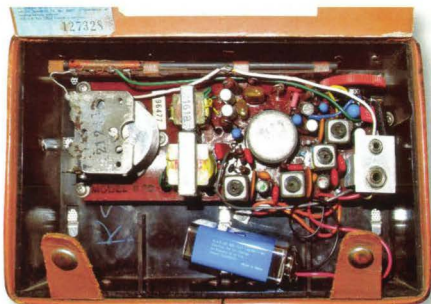
Most of the parts inside AWA B30 transistor radio are mounted on a densely-packed PCB. The original long 9V battery pack used in these radios is no longer available but a type 216 9V battery (wrapped in foam to stop it rattling) can be used instead.
