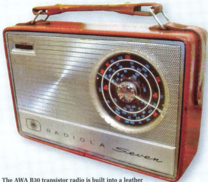
The AWA B30 transistor radio is built into a leather case and has just two controls: a large handspan dial and roller volume/power switch at top left.
