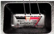
This photo shows the needle positions on the 'Radicator' for various signal strengths at 1400kHz & 600kHz.
