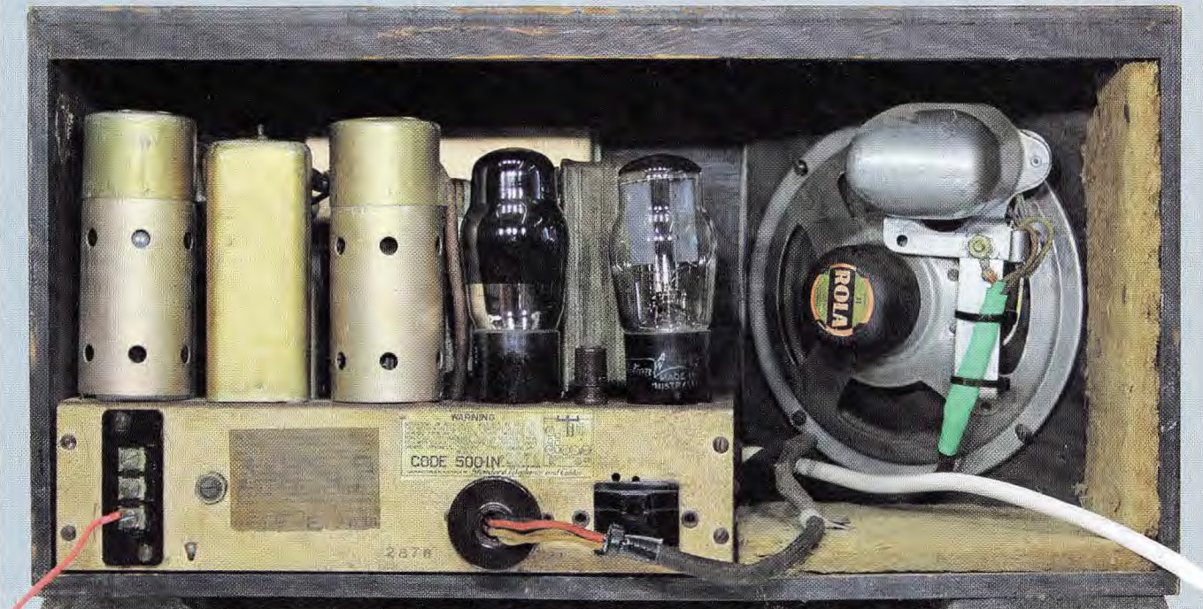
This view shows the Type 500A after restoration. The new 3-core mains cord bypasses the voltage selection plug (to the right of the loudspeaker socket) and is wired directly to the transformer. It also allowed the chassis to be safely earthed.
