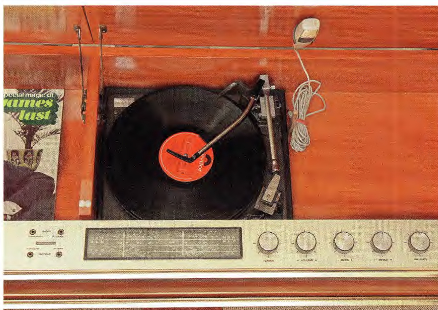
A BSR UA15 record changer was standard on the 11-102 but this can easily be upgraded to a Garrard AT6 as shown here. Note the microphone clipped to the underside of the hinged lid.
