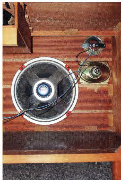
The 11-102 included two 12-inch woofers, two midrange drivers and two Magnavox E3.5 electrostatic speakers. The 11-103 used an extra pair of midrange speakers, bringing the total speaker count to eight.
