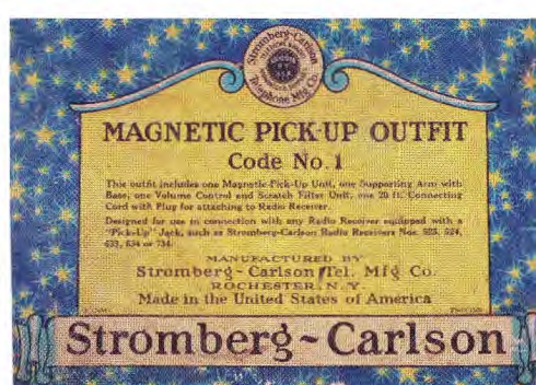
Stromberg-Carlson pioneered gramophone playback via a radio's audio amplifier stage. This photo shows the box-top of a 1928 add-on "Magnetic Pick-Up Outfit".
