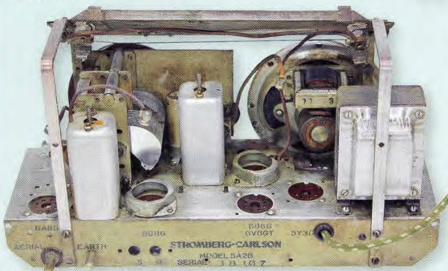
The chassis was given a thorough clean up with mineral turpentine to remove the wax and dust, while abrasive paper was used to restore the appearance of the aluminium IF-coil cans and the transformer covers.
