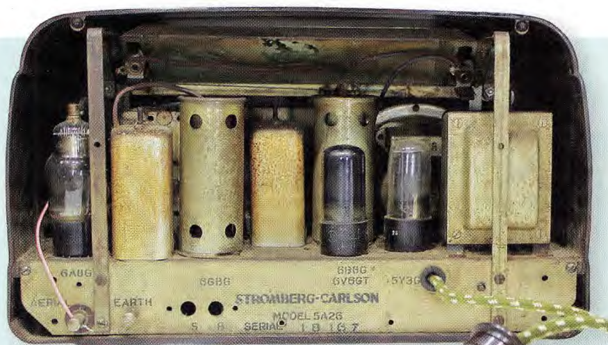
Above: the inside of the old radio looked like it had been splattered with fat but this "grease" probably came from the wax impregnation used in the power transformer and other components.
