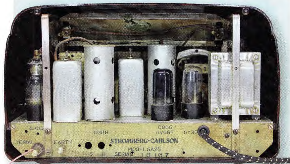
A new fabric-covered mains cord was fitted to the restored chassis. This was anchored using a cable clamp and its Earth wire secured to the chassis.
