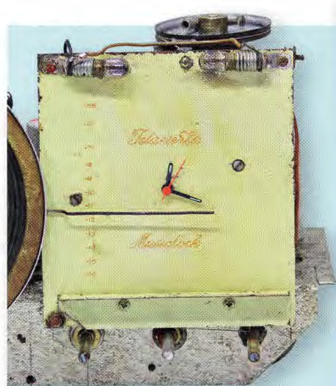
The clock face is positioned directly behind the dial which carries the hours and minutes markings.
