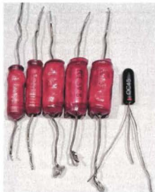
The electrolytic capacitors were all replaced, as was transistor TR2 which had excessive collector-base leakage.
