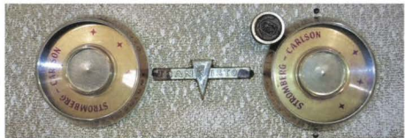
The controls for the Stromberg-Carlson 78T11/79T11 are mounted on the top of the case, with the volume control at left and the tuning control at right. The tuning wheel's rim is driven via a rubber grommet attached to a small knob.
