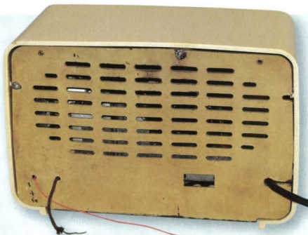
This rear view shows the Fleetwood 1003 fitted with its punched fibre-board cover. The two leads at lower left are for the antenna and earth connections.
