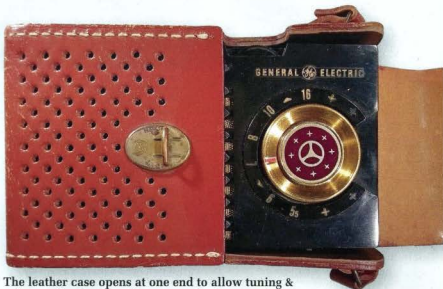
The leather case opens at one end to allow tuning & volume adjustments without completely removing the set.
