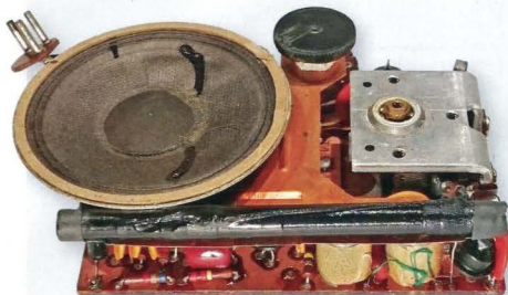
The GE 675 is built on a small double-sided PCB, with the ferrite rod antenna mounted along one side.
