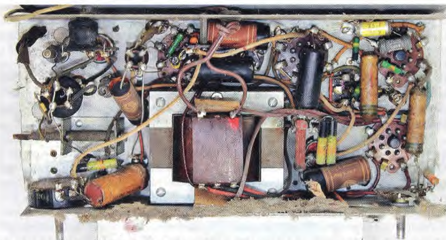
This view shows the underside of the chassis prior to restoration. Note the knot (now illegal) tied in the twin-flex mains cord that was originally fitted to the set. The volume control and several faulty electrolytic and paper capacitors had to be replaced to restore the set to operation, along with various other repairs.
