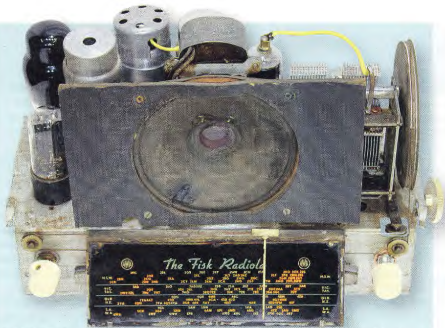
This is the fully restored chassis, ready for re-installation into its cabinet. In addition to the electrical repairs, the dial cord required restringing and a small tear in the speaker cone was repaired with PVA glue.
