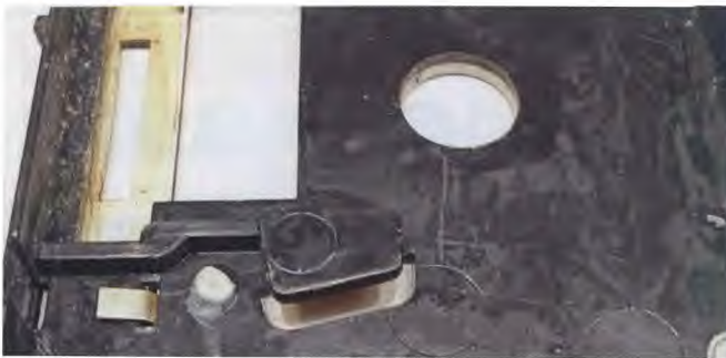
These two photos show the moulded plastic case lugs that are used to help secure the loudspeaker (left) and the chassis (above) – see panel.
