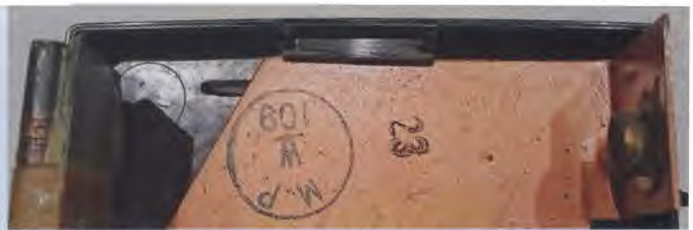
These two photos show the moulded plastic case lugs that are used to help secure the loudspeaker (left) and the chassis (above) – see panel.
