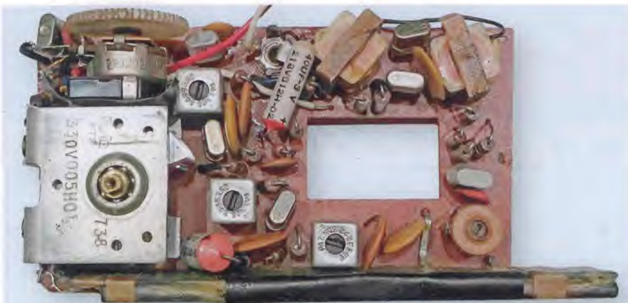
Above is another view of the top of the PCB, this time without the component labels. The layout is quite compact but the parts are all easily accessible once the metal shield and loudspeaker have been removed.
