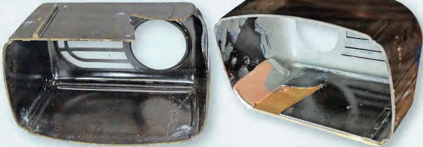
At left is another view of the damaged cabinet while the view at right shows the unit with repairs well under way. The bottom of the case was repaired by gluing a new base made from 3-ply under the existing base, while the hole in the side was filled using a section cut from a plastic cylinder. Car-filler “bog” was then used to fill the gaps.
