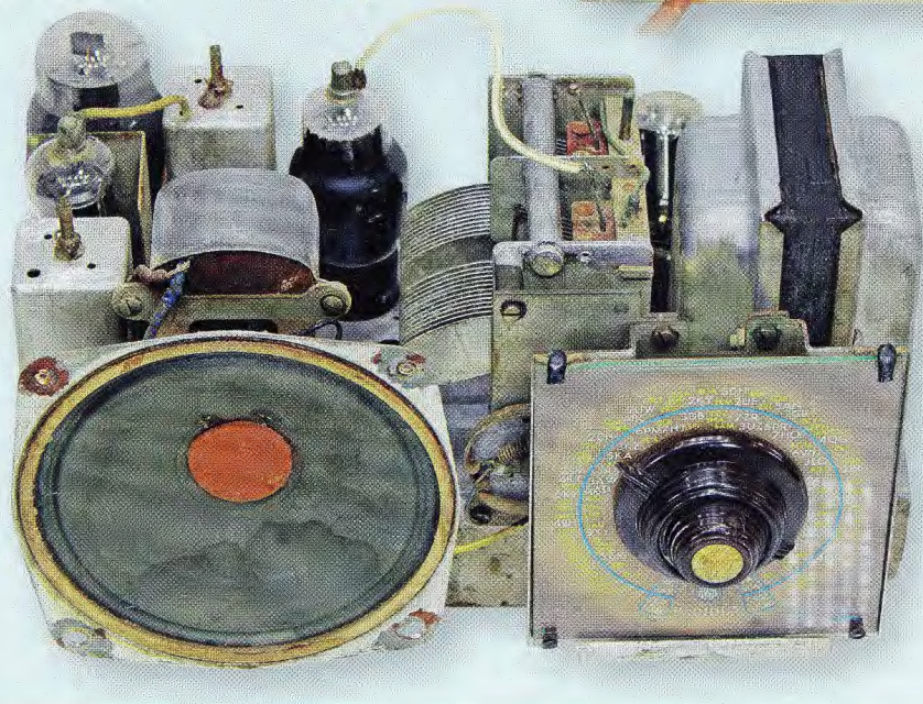
Below: a top-side view of the fully-restored chassis. An additional metal shield was later added adjacent to the 6G8 IF amplifier/detector valve to reduce the set's sensitivity to electromagnetic interference.
