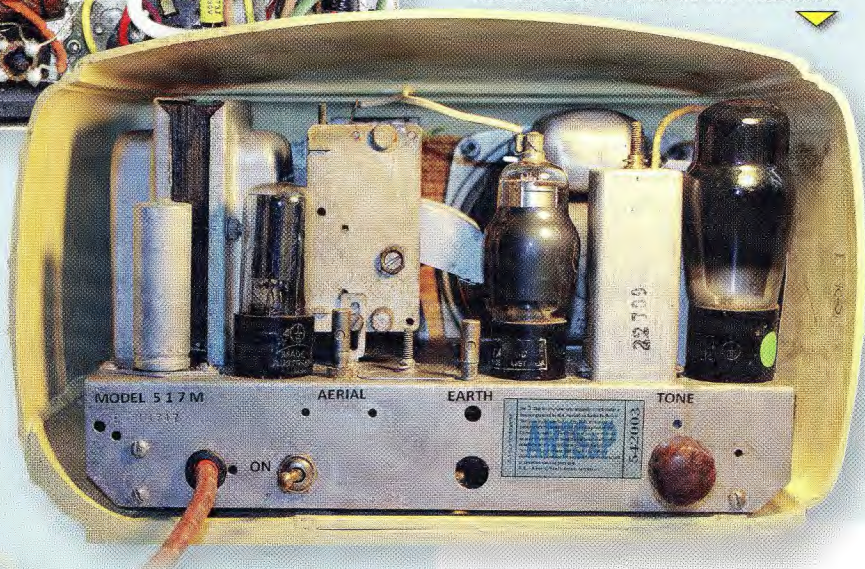
Below: the fully-restored chassis after it had been fitted into the repaired (and repainted) cabinet. The ARTS&P label was reproduced on a computer and printed onto an acetate transparency before being affixed to the rear of the chassis.
