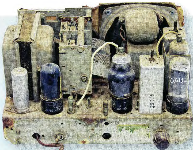
This view shows the top of the chassis before restoration. A 6AU4 had been fitted in place of the 6V6 output valve but it is completely unsuitable for this role since it is a half-wave rectifier.
