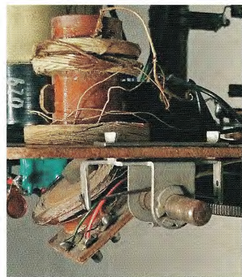
This shaft (left knob) varies the coupling between the primary and secondary aerial coils to provide the volume control.
