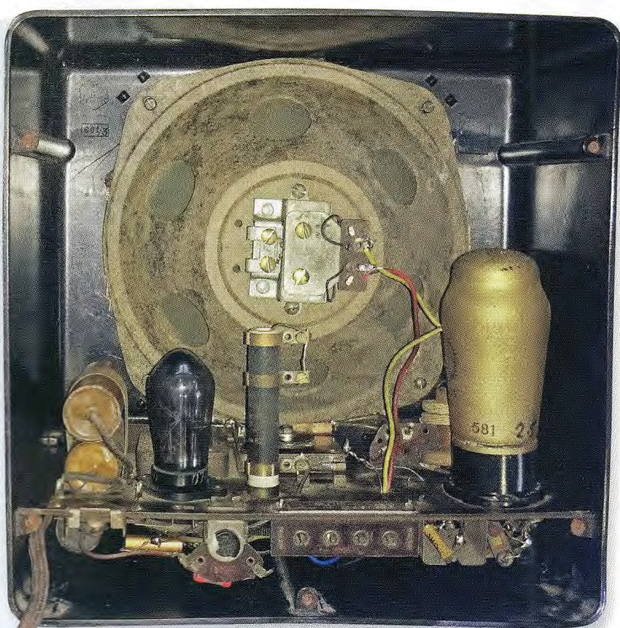
The DKE38 shown with the original moving-iron loudspeaker. Note the vertical tapped resistor which is used to set the filament current in the rectifier and the triode-tetrode. The preset control is R6 which was adjusted by the factory to set the back bias for the tetrode section.
