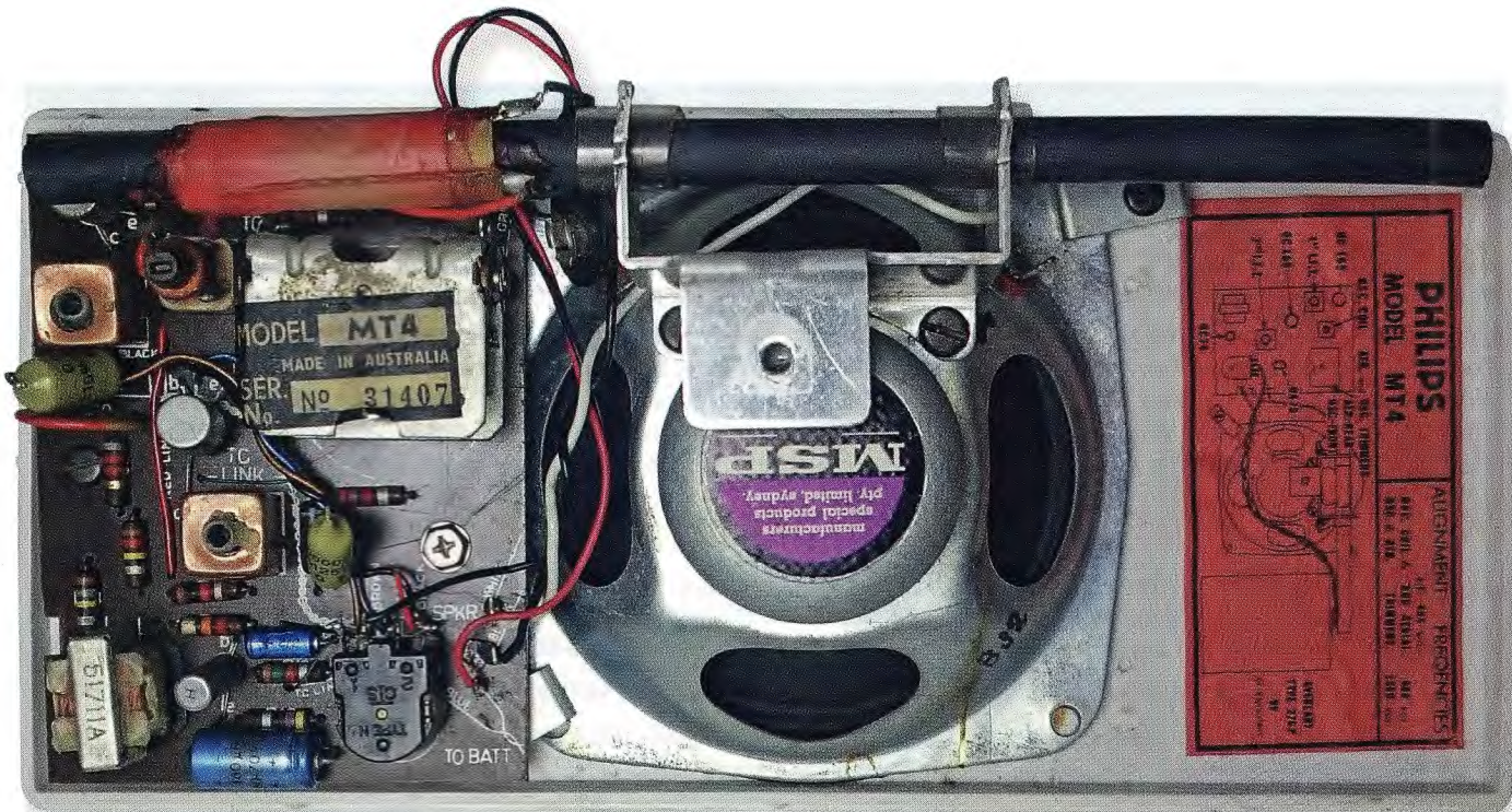
The Philips MT4 was equipped with a full-size ferrite rod antenna which ensured good signal pickup. The PCB on the left was quite compact given the relative complexity of the circuit. The large space on the right accommodated the Eveready 276P battery which gave somewhat more than 100 hours of life.
