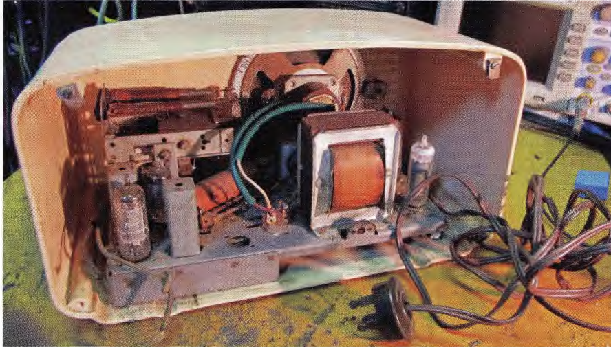
The inside back of the Astor HNQ. The damaged 6AQ5 output audio amplifier valve is directly right of the power transformer. The visible two-core power cable was replaced with a proper three-core cable with Earth.
