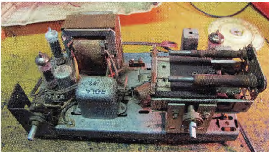
The contacts on the power switch/volume control (bottom left) were badly corroded; a bit of cleaning brought it back into action.
