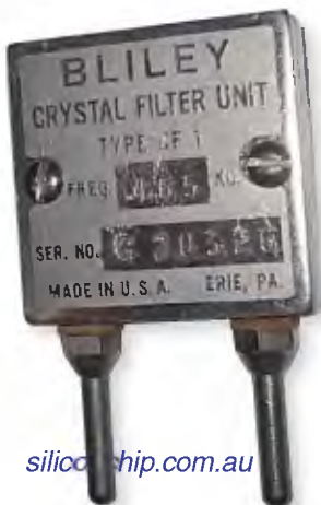
The Bliley 465kHz crystal filter is shown enlarged for clarity, with an actual size of 30 x 40mm. Serial number: G20326.
