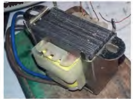
A Jaycar Cat. MM2007 transformer was rewound to act as the matching transformer for the speaker unit.
