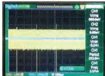
Fig.5: with the Lamb Silencer switched out, spark interference is visible in the output.
