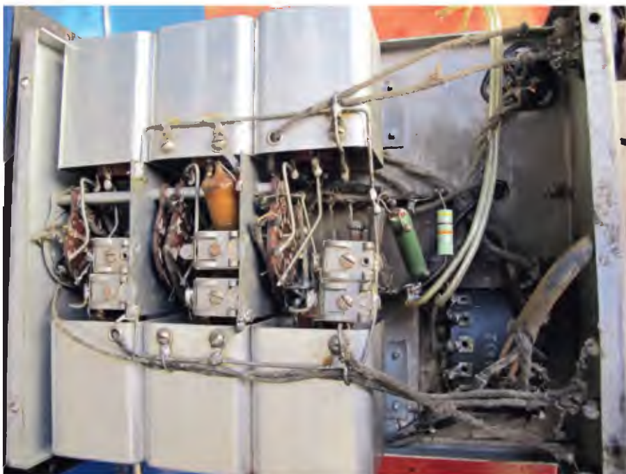
Left: the original underside of the DB-20 pre-selector. The DB-20 provides continuous coverage from 550kHz to 32MHz in six bands, and has a gain of ~20-25dB which is the basis for its name. The DB-20 was also used by the US Navy under the name CME-50063.
