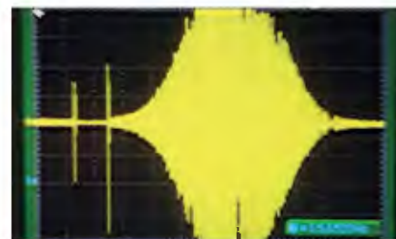
Fig.2: an IF pass response without the Bliley crystal filter
