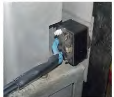
Below: a replacement switch for gain control "A" on the front panel.
