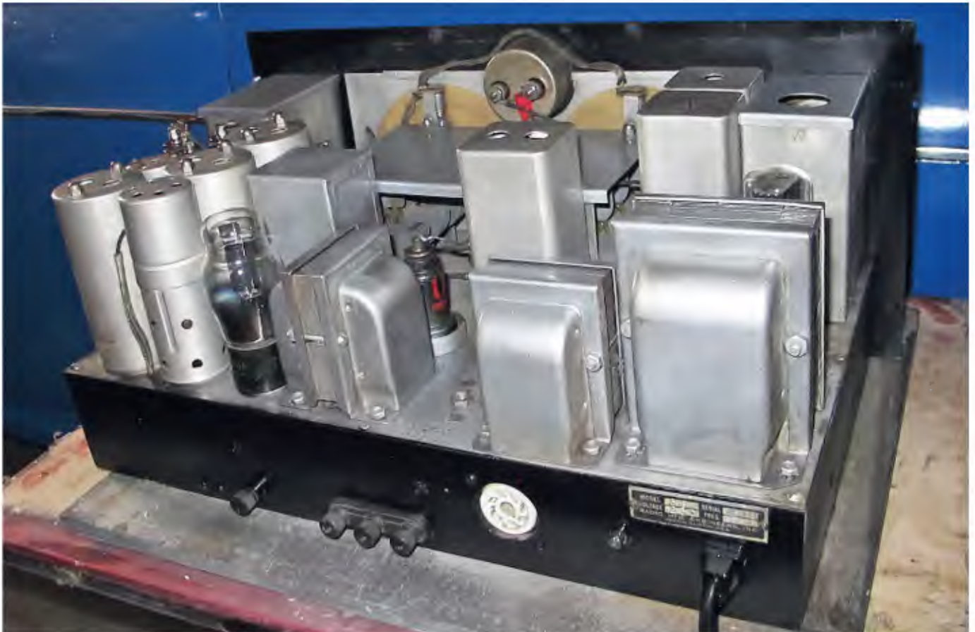
The 'restored' underside of the chassis can be seen above, with the topside shown below. This receiver was manufactured by RME at 306 First Avenue, Peoria, Illinois USA as stated on the label on the rear of the set. Around 1953, RME merged with Electro-Voice who are still around today.
