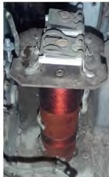
Above: the underside of the RME chassis before any restoration work was done. Right: the calibration trimmers inside the broadcast coil had their screws unwind over time due to vibration.
