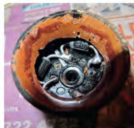
A 5V4 valve envelope was used as a dummy with 1N4004 diodes installed in its base. This acted as V4 while retaining a 'vintage' appearance.
