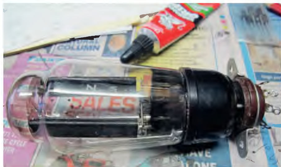
A 5V4 valve envelope was used as a dummy with 1N4004 diodes installed in its base. This acted as V4 while retaining a 'vintage' appearance.
