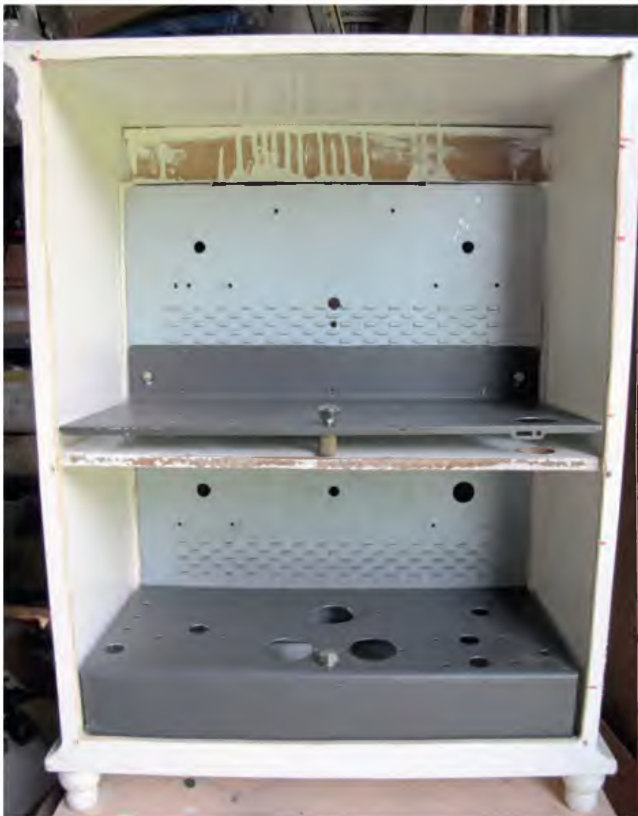
The chassis was made from an old computer case and holes were marked and drilled for the various component locations.
