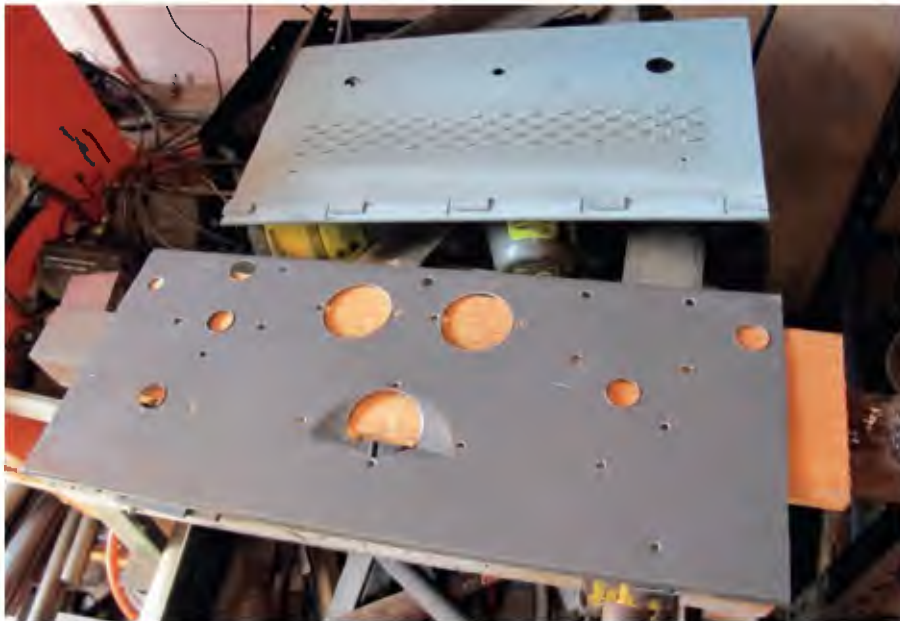
The chassis was made from an old computer case and holes were marked and drilled for the various component locations.
