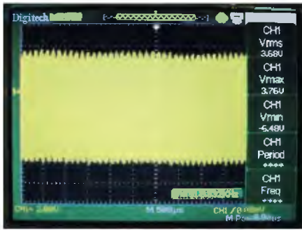
Fig.2: the detector plate (V1) was fed with a 915kHz sinewave, showing just the carrier signal.
