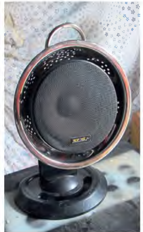
The completed tabletop speaker. It consists of a computer monitor stand, colander, and an old car speaker. Like the rest of the design, it's a hodge-podge of parts.
