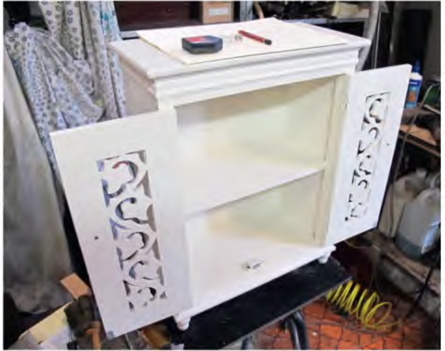
The cabinet was based on a two-door utility cabinet that had been left out in a council clean-up. The top shelf would house the RF, tuning and detector sections while the bottom would be for the power supply and audio valves.
