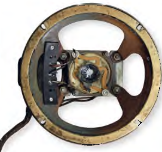
The 7-inch (178mm) electrodynamic speaker was missing its cone. A ferrite-magnet 4Ω speaker was instead placed inside the area where the cone would normally be as shown in the adjacent photo.
