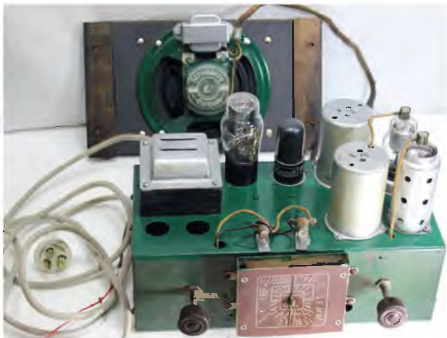
The 7-inch (178mm) electrodynamic speaker was missing its cone. A ferrite-magnet 4Ω speaker was instead placed inside the area where the cone would normally be as shown in the adjacent photo.
