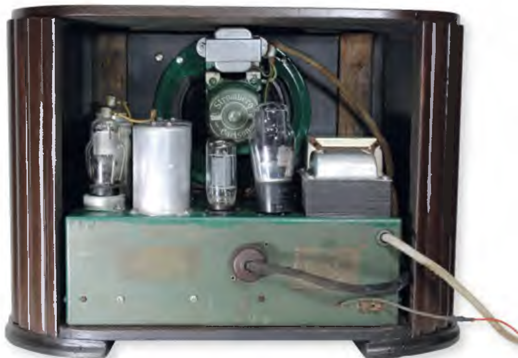
On the rear of the chassis you can see the cloth-bound mains lead which was a replacement for a figure-8 flex as a way to Earth the chassis.
