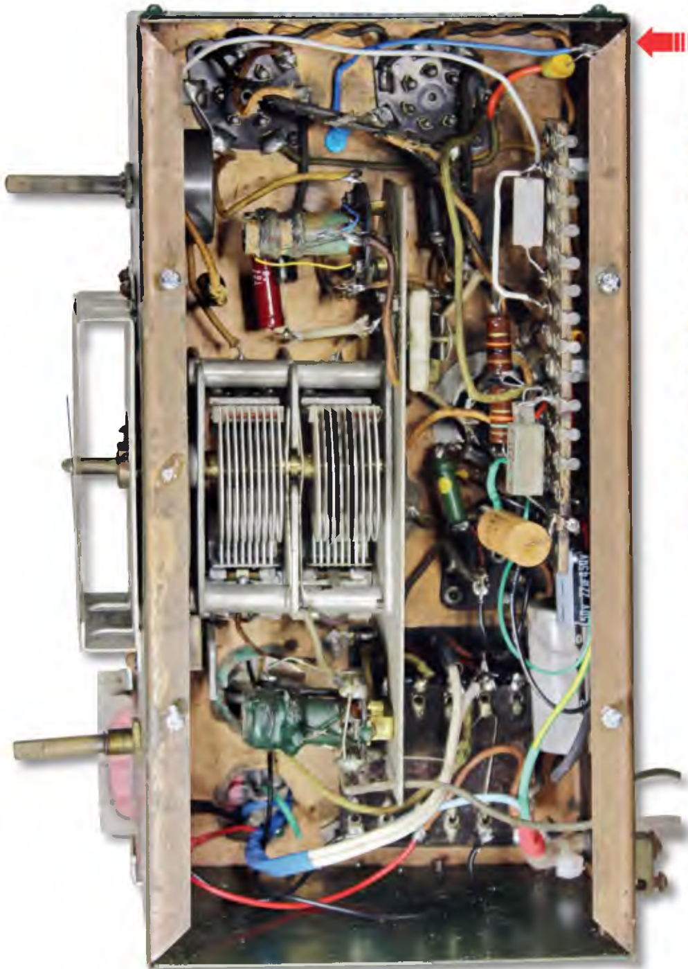
Shown at left is the underside of the chassis after restoration. A subsection is shown above of the green multi-section wire-wound resistor which was replaced with a tag board.
